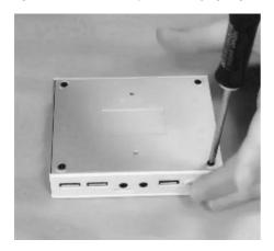
mSATA, SIM socket, miniPCIe and battery which are located at the bottom side of the motherboard are now accessible for installation/replacement.
