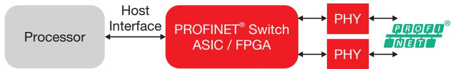
Figure 4: PROFINET switch with ASIC and external processor
